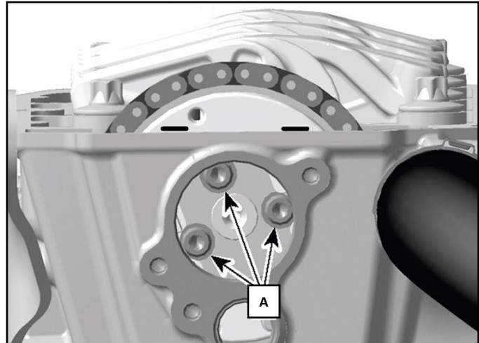
Replace engine blow-by valve. **NOTE: BRP recommends replacing blow-by valve v-ring. Apply engine oil to o-ring, v-ring & thrust washer. Apply Loctite 243 to bolts. Torque to 6 ft•lb (9 N•m).**
