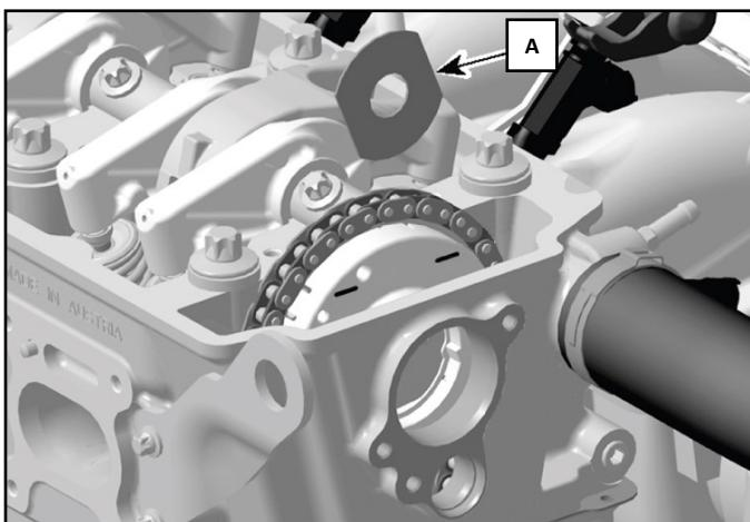
Three bolts (A) secure the cam gear to the cam shaft. Remove and replace 1 bolt at a time. **NOTE: Apply Loctite 243 to bolts. Torque to 12 ft•lb (16 N•m).**
